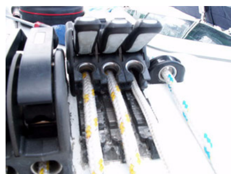
Pass the rope through Reassemble the clutch following the reverse of the dismantling procedure
