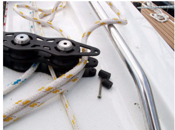
Pass the rope through Replace the screw and the 2 spacers
